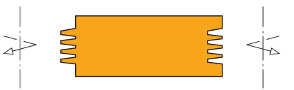
Profile 3 with shoulder cutters on the same level
