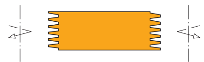
Profile 1 with continuous finger jointing
