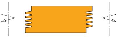
Profile 2 with staggered shoulder cutters
